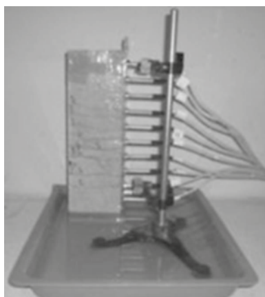
Figure 5. Photograph of water uptake experiment
