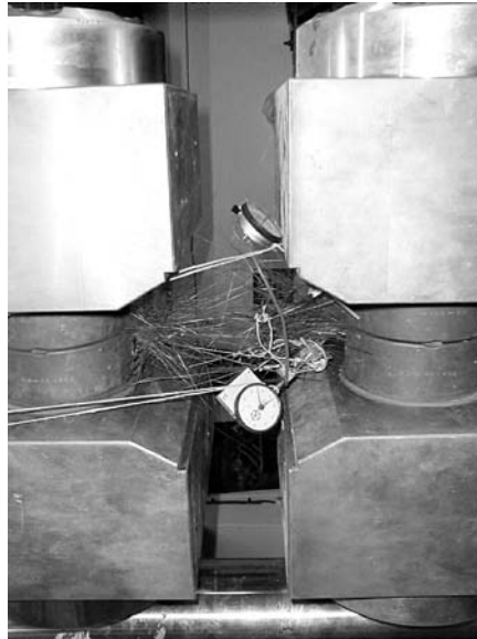
Figure 4. Explosive failure of the standard carbon fiber specimen tested
