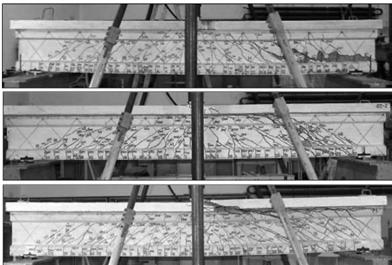
Figure 9. Shear failure. From the top: beam ST1 – failure of the web, beam Z2 – combination of failure web/contact, and beam D2 – failure in the contact gap
